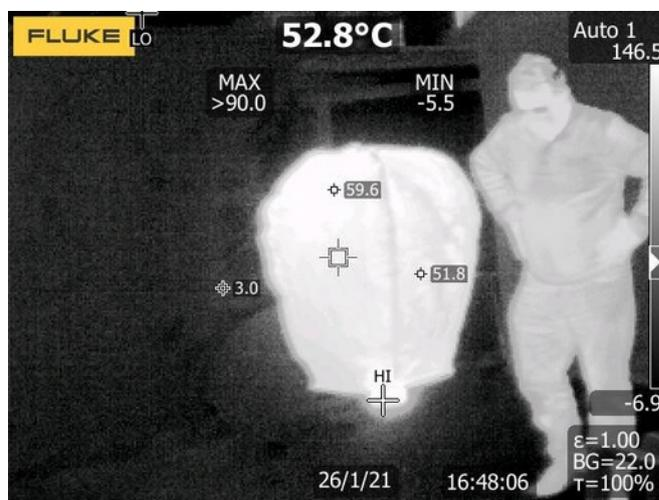
**Fig. 29 – On left : example of band 3 IR image – On the right : thermo point image ; the temperature displayed at the top ( $52.8^\circ\text{C}$ ) corresponds to the center of the image, the 3 measuring points on the periphery give an idea of the dispersion**
