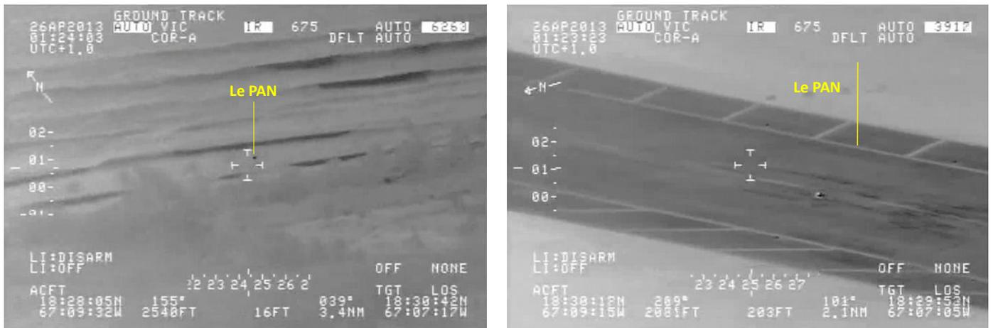
**Fig. 7 – On the left view, the target distance is 6300 m, the calculated size is 1.2 m – For 3900 m (right view), the size is 1.3 m, confirmed by comparison with the width (45 m) of the central strip of the runway – the maximum size is that of an object close to the target i.e. close to the ground.**
