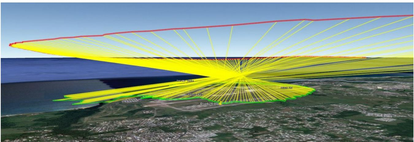
**Fig. 12 – In red : trajectory of the DHC-8 ; in green : the target positions ; in yellow : the lines of sight**
