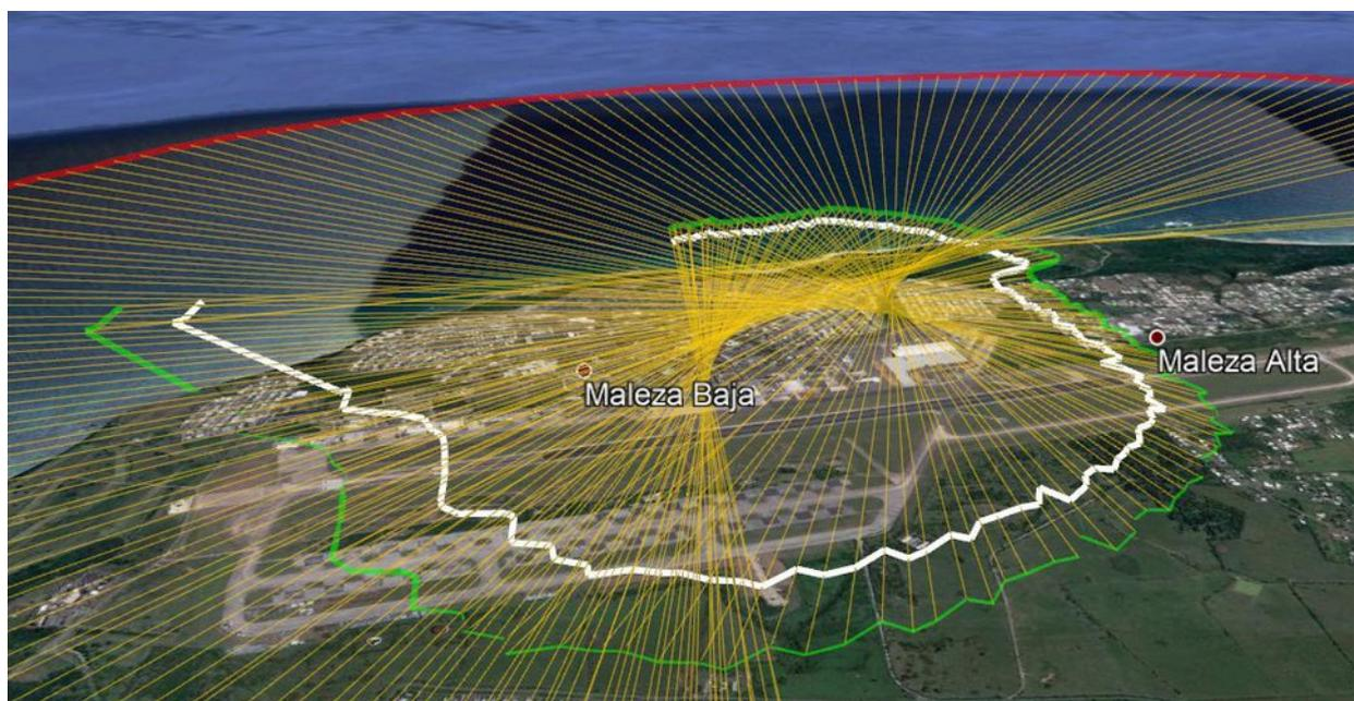
**Fig. 18 – In white line : UAP trajectory in terrain following mode,  $Z = 100$  ft**
