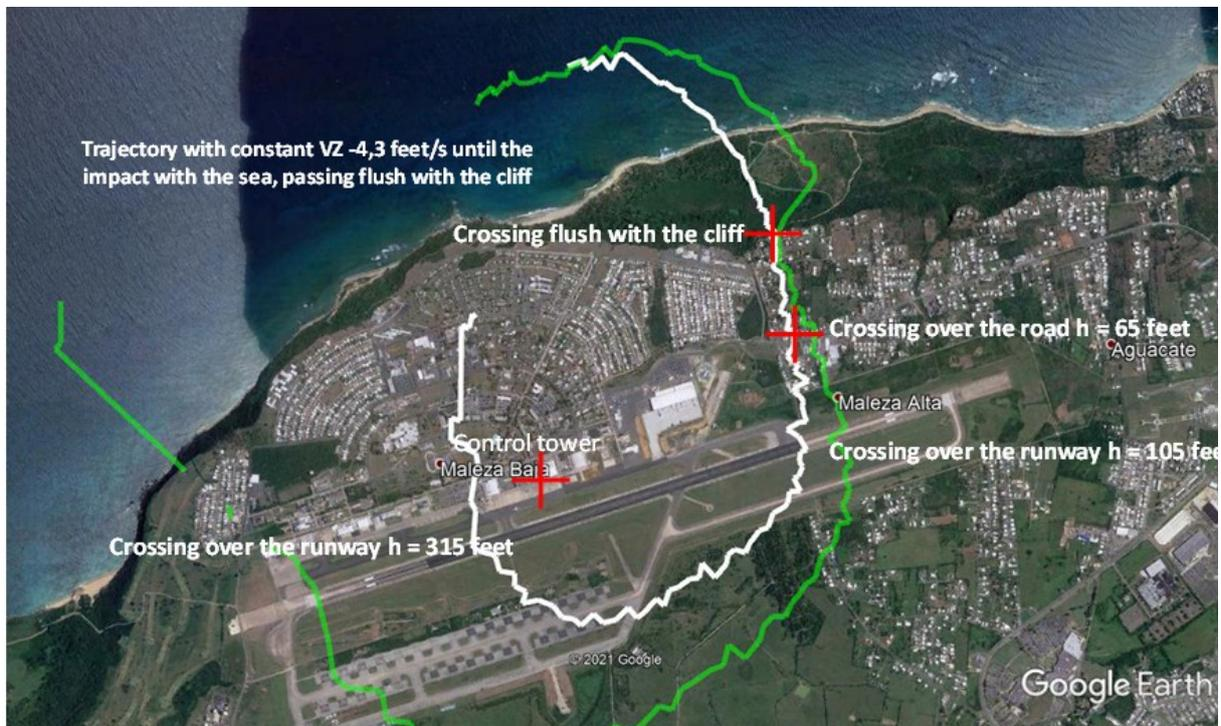
**Fig. 23 – UAP trajectory for  $VZ = -4.3$  feet/s**
