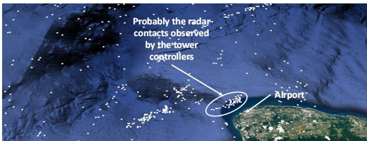
**Fig. 3 - Primary radar contacts from 20:58 to 21:26 LT (white dots)**
