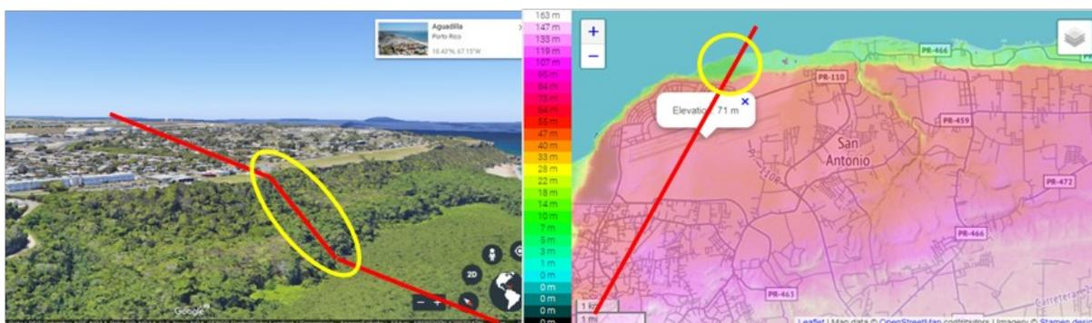
Fig. 14 – The steep slope of the terrain at the passage of the coast causes the important change of position of the point targeted by the camera and therefore of the laser distance
