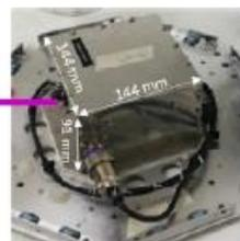
Robust interferometric interrogator
