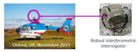
Shape change data was acquired and streamed while blade rotated at 380 rpm during several ½ hour trials
