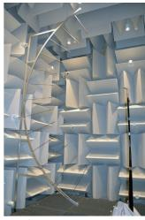
Characterization of low Reynolds number rotors in an anechoic room. © ISAE-SUPAERO
